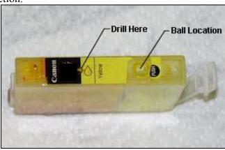
2. Use our black tool and a small hammer or equivalent device to push the ball into the reservoir. It does not take much, just one sharp blow right on the plastic ball. (See step 9 for alternative.)
